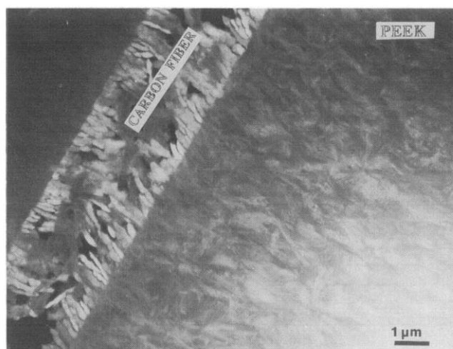
Figure 1 Spherulites at the interface in an A specimen ( T_m=360^\circ\text{C} , T_c=310^\circ\text{C} ). Transmission electron microscopy, dark field image
